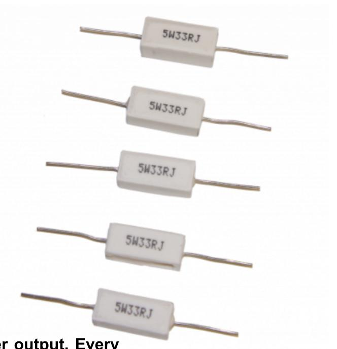
Connect one resistor in parallel across the positive and negative of each speaker output. Every output MUST have a resistor in order for the head unit to output sound. If you STILL do not have sound you will need to connect TWO resistors in parallel and then connect that across each output.
