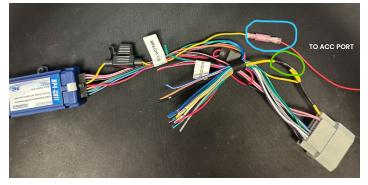
STEP 3 – Remove HVAC control panel shown below. Route the wire from the RP4-CH11 harness to the accessory port on the driver side of the HVAC control panel as shown below.
