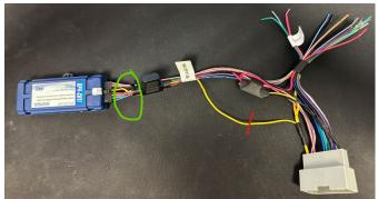
STEP 2 – Tape the vehicle side of the constant wire off safely (GREEN). Route a wire to the module side and run down the dash to the accessory port. (BLUE)
